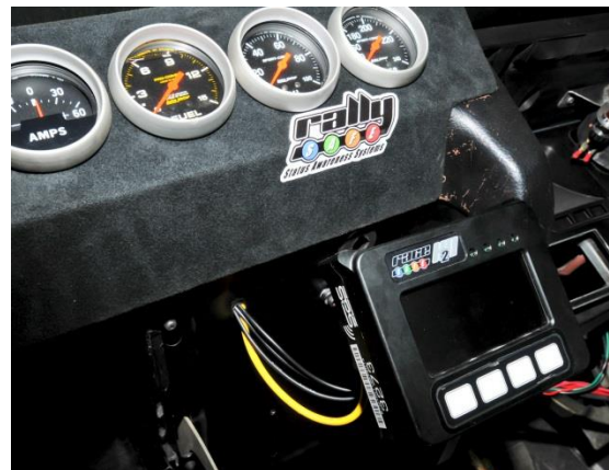
The RallySafe unit then mounts to the 25mm Rubber Ball mount. (This is connected through the RallySafe connector)
