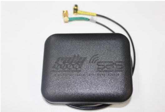
A minimum of 300mm of Rallysafe Power Supply Cable and Antenna Leads should be left at the unit mounting bracket location for connection to the unit
