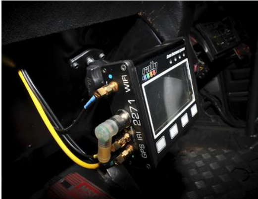
Here is what a standard installation would look like. Note the unit and aerial placed in clear and unobstructed view.
